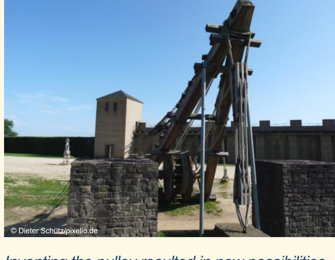
Inventing the pulley resulted in new possibilities. Without the pulley and crane the Colosseum in Rome could have never been built. (Replica of a Roman crane in Xanten)
